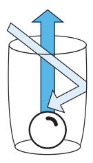
Result: Less pressure on the top of the ball forces it upward
